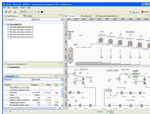
**Figure 1.** Apros 6 process simulator, integrated in Simantics Workbench.
