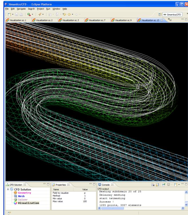
Figure 7. Stream lines visualization in a pipe.
