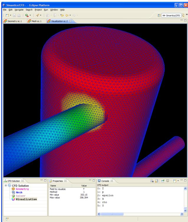
Figure 5. Mesh and surface plot of temperatures in the tank.
